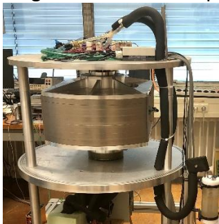
(Left) Magnetocaloric heat pump and (right) 3D printed magnetocaloric materials
